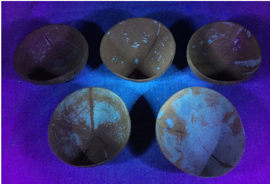
Fig. 4: Interior of coconut bowl samples (Group 1) viewed under UV light ( \lambda_{exc} = 365 \text{ nm} ). UV-induced visible fluorescence image was taken with an iPhone to capture fluorescence colors visible to the naked eye.
