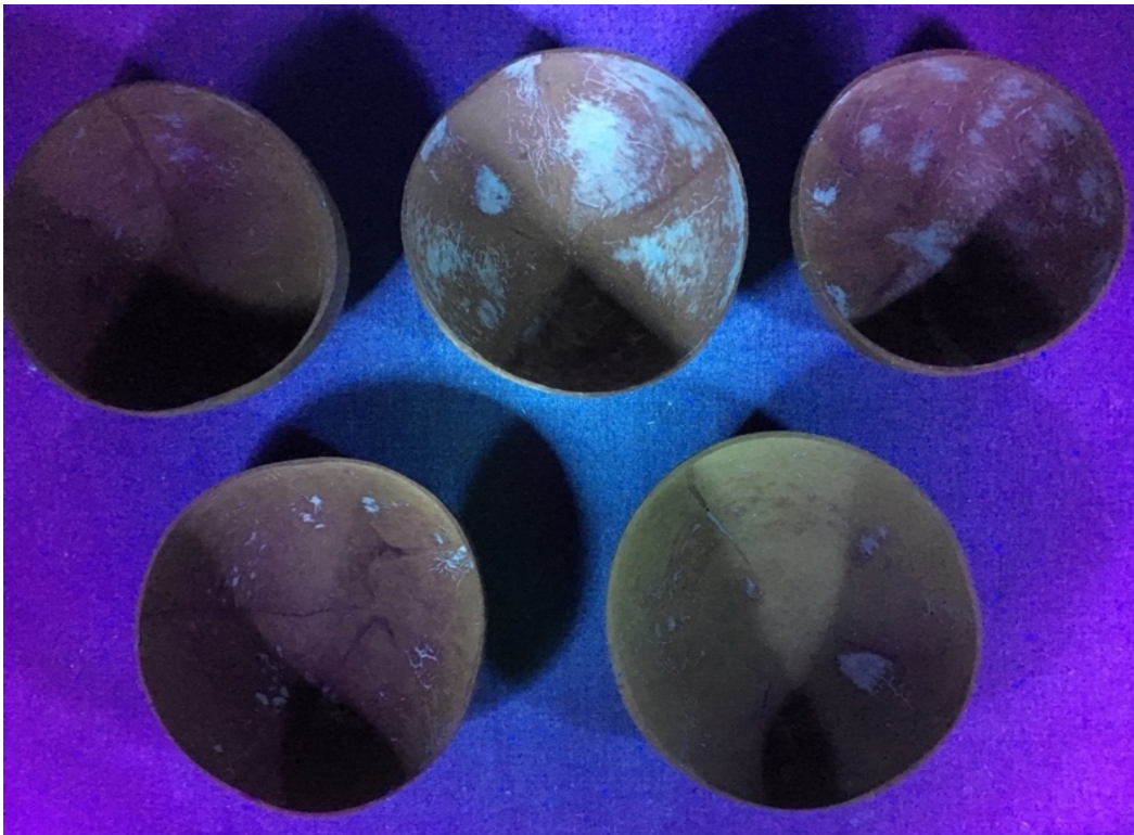
Fig. 8: Interior of coconut bowl samples (Group 2) viewed under UV light ( \lambda_{exc} = 365 nm). UV-induced visible fluorescence image was taken with an iPhone to capture fluorescence colors visible to the naked eye.
