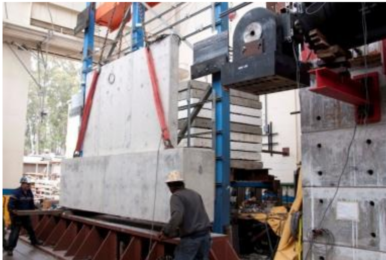
Figure A.15: Lowering the First Wall into the Testing Location
