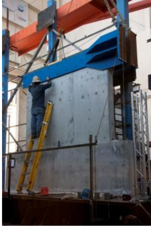
Figure A.16: Attaching Loading Plate to Wall
