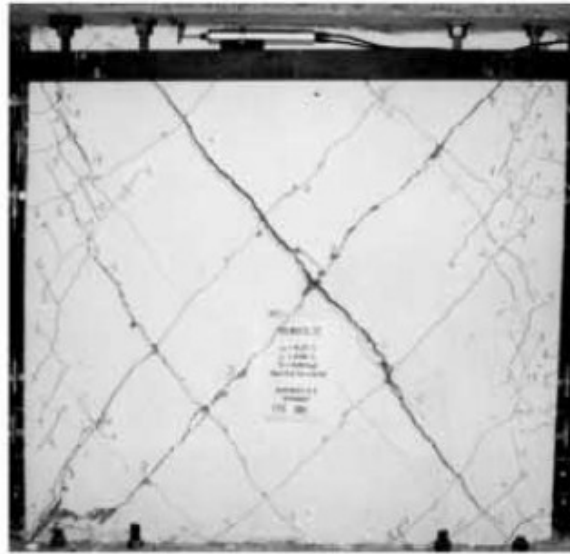
Figure 2.1 Diagonal Tension Failure (Gulec 2009, from Hildago 2001)
