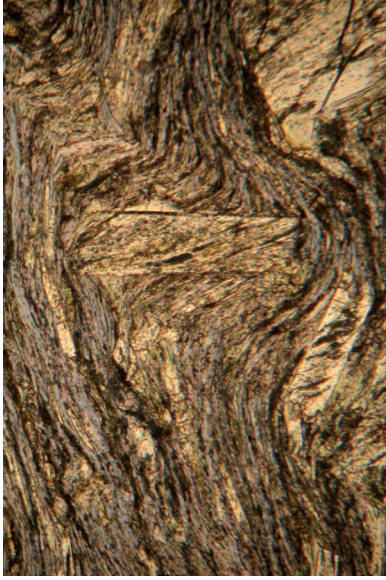
Figure 11. Photomicrographs from the same thin section of lawsonite-blueschist metabasalt at Diamante. In the image on the left, a top-to-the-right shear direction is visible. In the image on the right, top-to-the-left CS' shears can be seen. Both images are roughly 200 \mu\text{m} across. Images were taken by Francesca Liberi.
