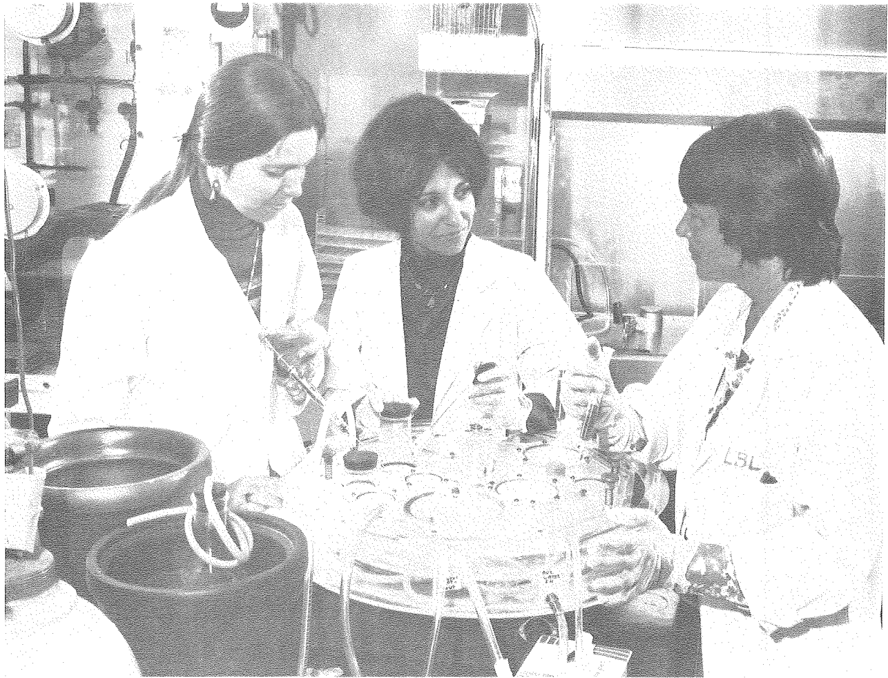
Figure 1. The steady-state apparatus for animal cells in culture was designed and built in this laboratory. Up to 30 replica plates may be kept under constant temperature and pH for kinetic tracer studies. (BBC 765-4658)
