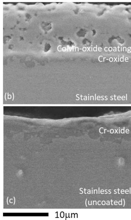
Figure 2. Oxidation behavior. (a) Intermittent weight gain data for coated (filled markers) and uncoated (open markers) coupons at 800 °C (circles, squares) or 850 °C (triangles) in humidified air (circles) or humidified O 2 /N 2 (30:67) (squares). SEM cross section images of (b) coated and (c) uncoated samples after 500 h oxidation at 800 °C in humidified O 2 /N 2 (30:67).
