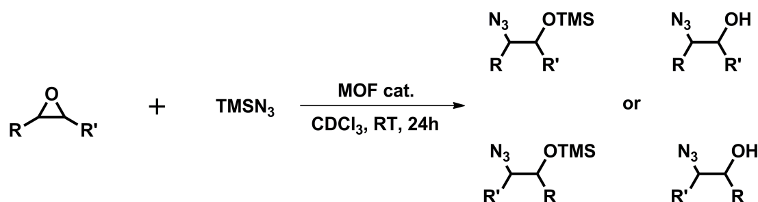
Scheme 5-3. MOF catalyzed epoxide ring opening reactions with \text{TMSN}_3 as the nucleophile.
