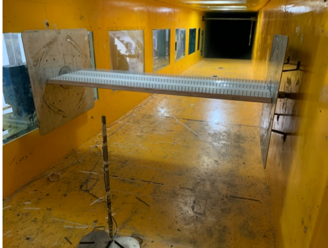
Figure 3-1-6: Set-up of the aerostatic coefficients test
