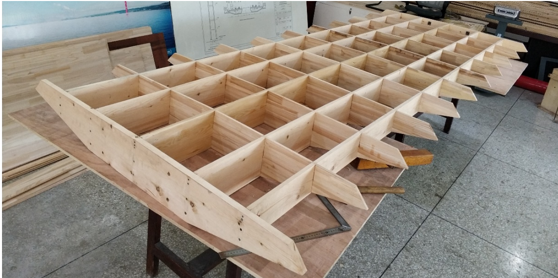
Figure 3-3-2: Internal structure of the girder section
