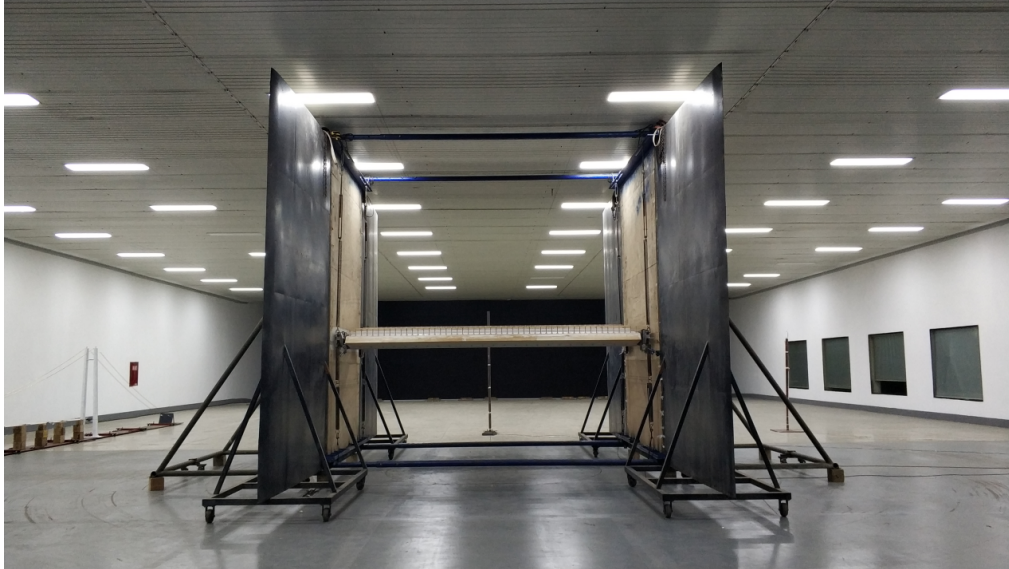
Figure 3-3-6: 1:20 girder section experiment setup
