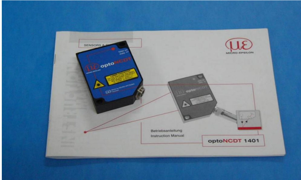
Figure 3-3-8: LASER transducer used in the experiment
