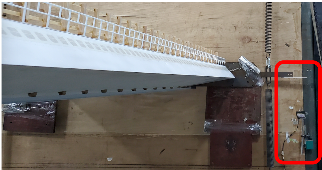
Figure 3-3-9: Location of LASER transducers
