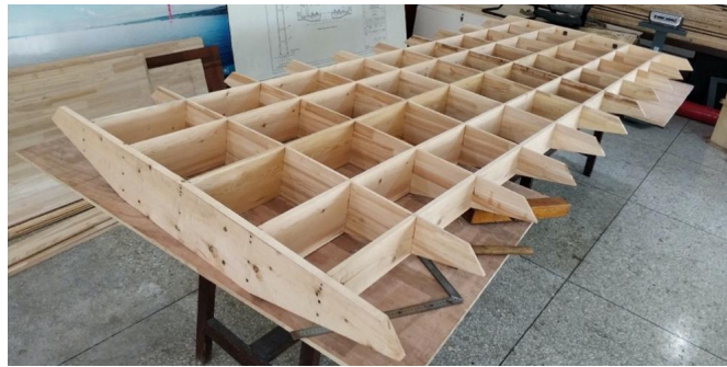
Figure3-1-1: Inner structure of the girder section
