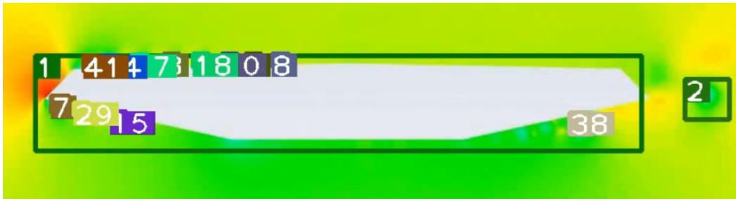
Figure 3-2-10: Tracking result for the streamlined girder section
