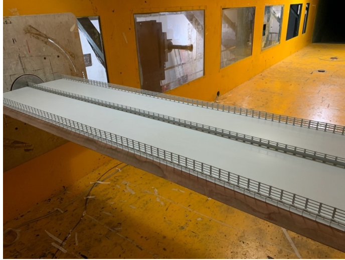
A- 1: 0.67m central stabilizing boards
