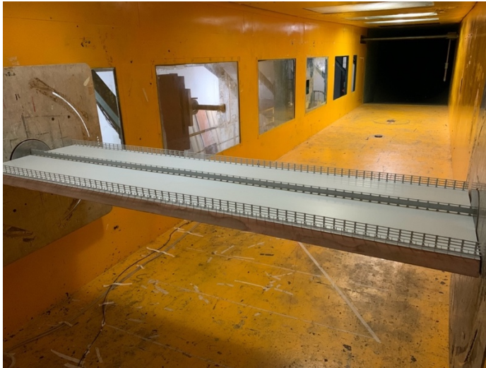
A- 2: 1.02m central stabilizing board
