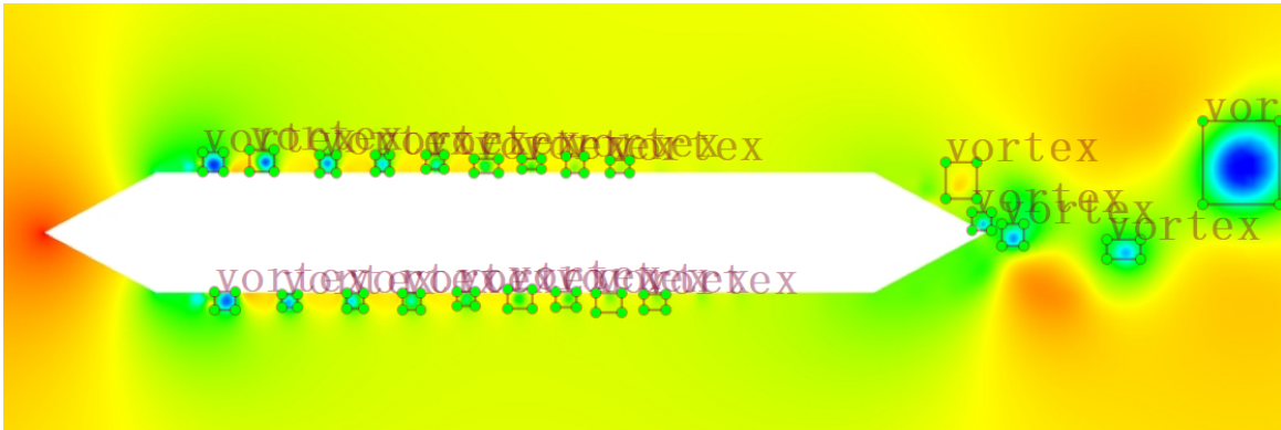
Figure 3-2-4: Vortexes labeled in the flow field
