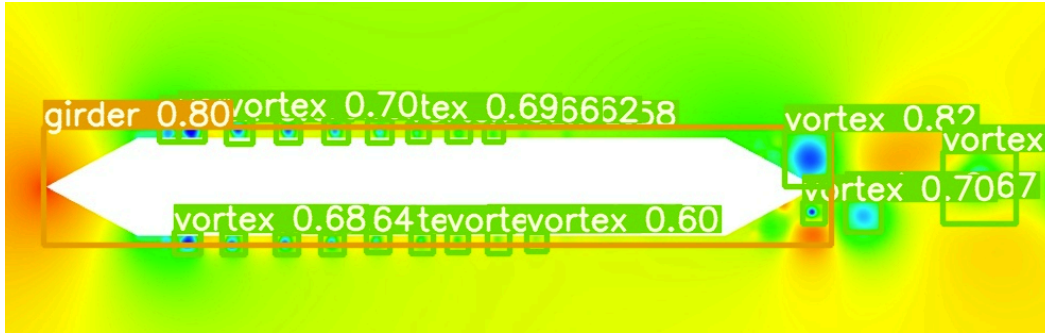
Figure 3-2-7: Recognition results for the 1:6 rectangular section with wind noses
