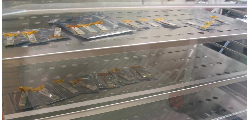
Figure 5.8: A picture of 19 of the 20 tested modules in the nitrogen storage chamber.
