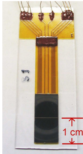
Figure 3.42: Picture of two silicon chip PSAPDs (black squares) on one flex cable (yellow material). The module is mounted to glass with tape to rigidly secure the structure during movement and coupling to acquisition electronics.
