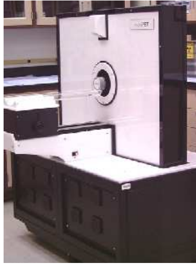
Figure 6.4: A picture of a small animal imaging system with a grey and white phantom resting on a clear test bed.
