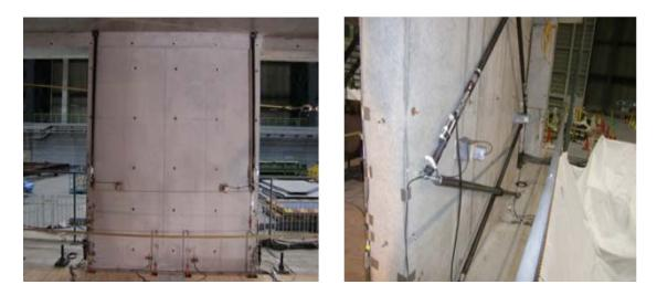
Figure 5-9. Instrumentation of the RC shear walls
