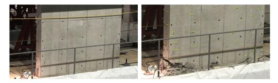
Figure 5-16. Damage on the RC shear walls (Axis A) at (a) 50%, (b) 100% Kobe record
