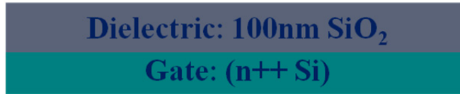
Figure 13. The cross section of the TFT structure at the end of step1.
