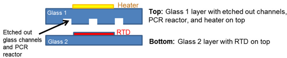
Figure 84. Another cross-section of the microfluidic chip.
