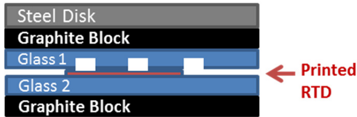
Figure 87. Wafers and graphite blocks set up for thermal bonding.
