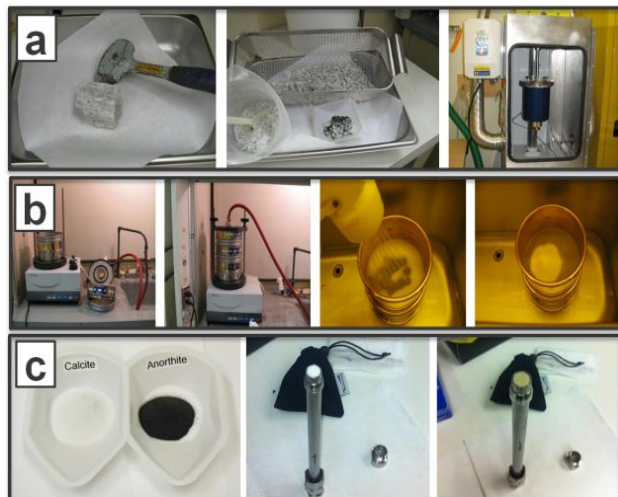
Figure 2 – CF sample preparation workflow. Grinding (a), wet-sieving (b) and column-packing (c).
