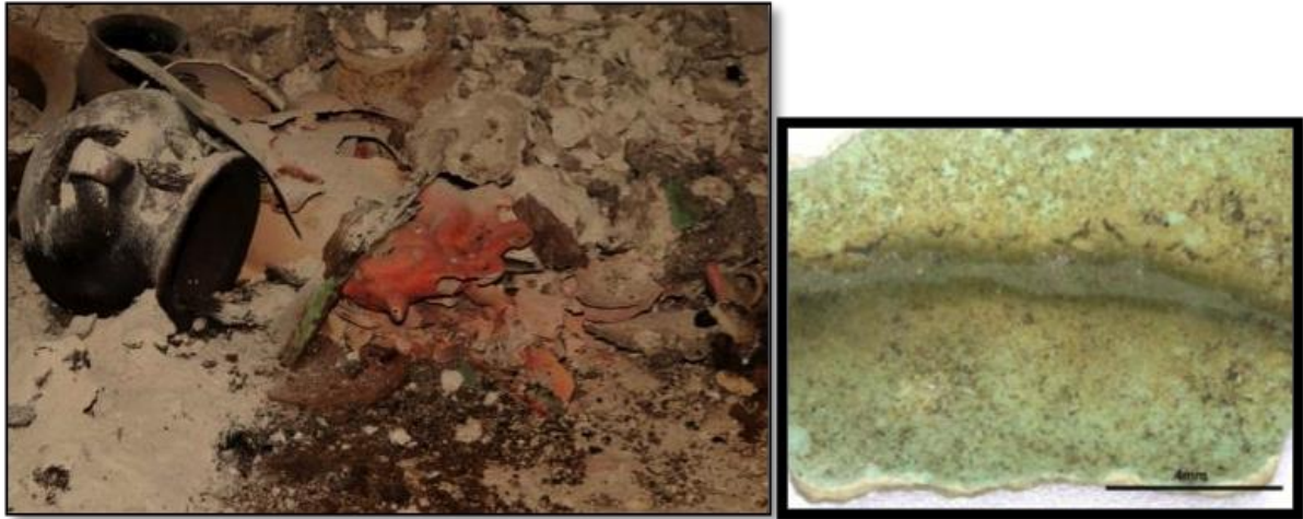
Figure 15. SAMPLE 09: Green painted stucco fragments. Stereomicroscope observations: top side – green paint and brownish yellow debris on the top; dark green line across green surface with corresponding darker brown line on back side of fragment; bottom side – whitish layer; plaster-like.
