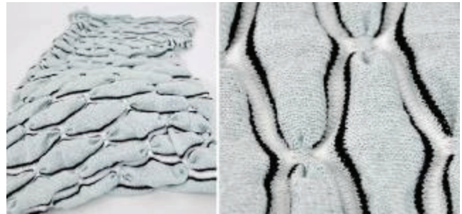
Figure 3. Integrating conductive yarns for sensing.
