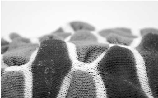
Figure 4. Experimenting with coatings for air tightness.
