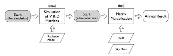
Figure 1. Simulation process flow chart
