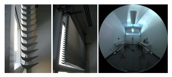
**Figure 2.** (left): Side view of the OLS on the inward face of the clerestory glazing. (middle): Oblique view of the OLS. (right): Photo of the test space with OLS installed (looking from the back of the space towards the window)
