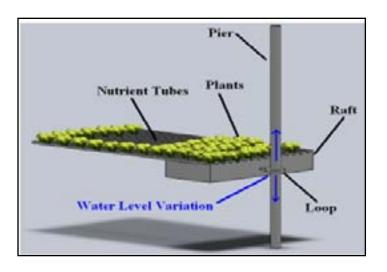
Figure 4. Schematic of anchoring system (not to scale).
