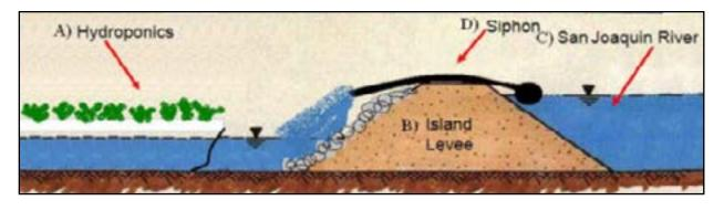
Figure 3. Flood management zone during high water event.
