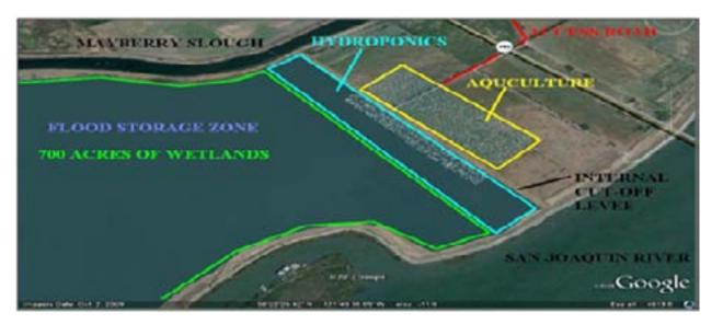
Figure 2. Water management system layout.
