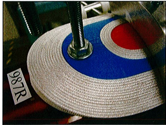
Figure 4: A practice coil using rapid-prototyping parts.
