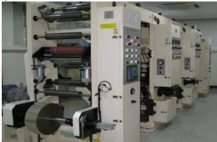
Figure 2.4. A laboratory scale gravure printing press with two print units, and automatic registration capability.
