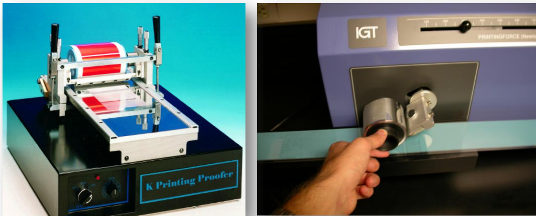
Figure 2.3. Two proof presses. A K printing proofer (left) and a IGT G1-5 (right).
