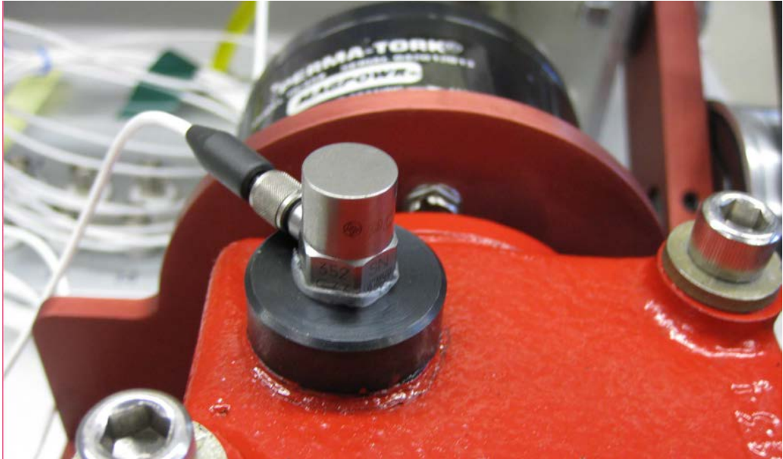
Figure 13: Gear Box Sensor Location (Channel 1)
