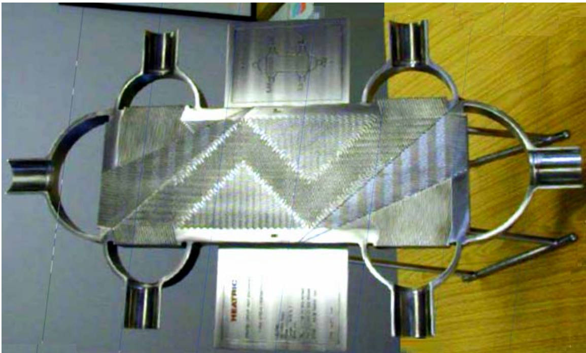
Figure 0-2: Photo of a cut-away model of a typical Heatric plate-type compact heat exchanger showing multiple inlet and outlet manifolds and slices across various plates and flow channels.
