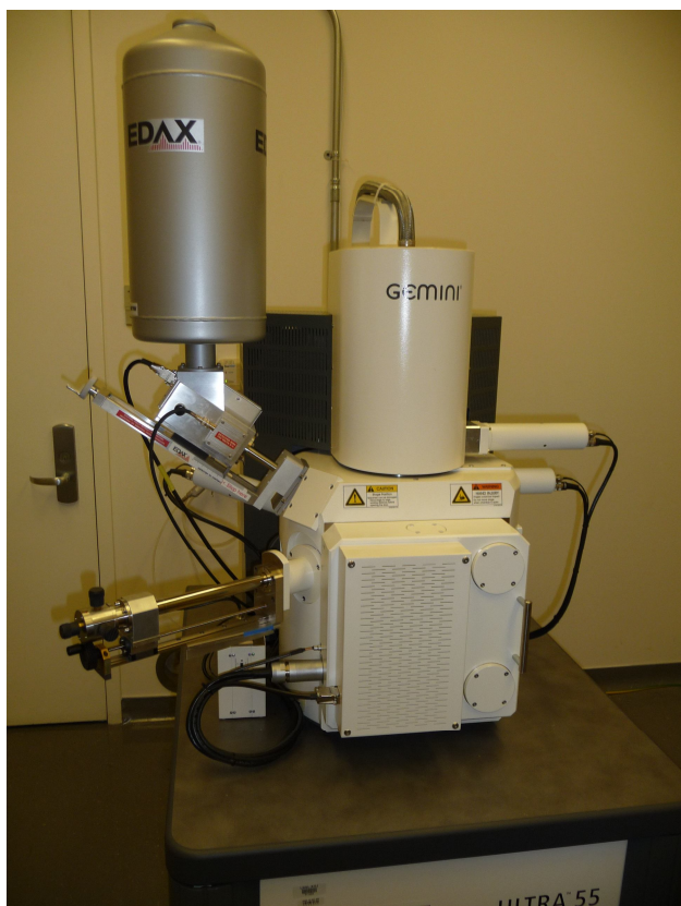
Figure 3.3 Zeiss Ultra 55 Field Emission SEM at Lawrence Berkeley National Laboratory's Molecular Foundry
