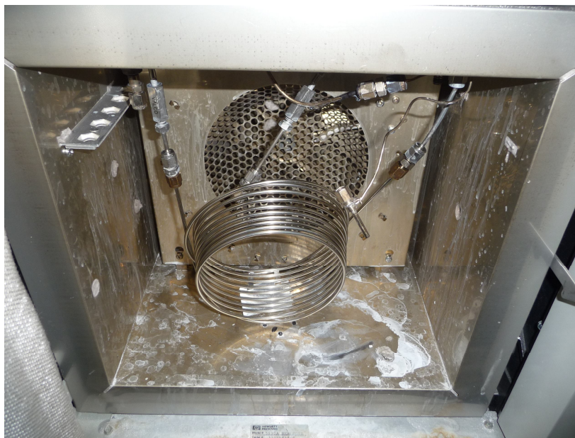
Figure 4.2 Packed column inside the oven of a GC.
