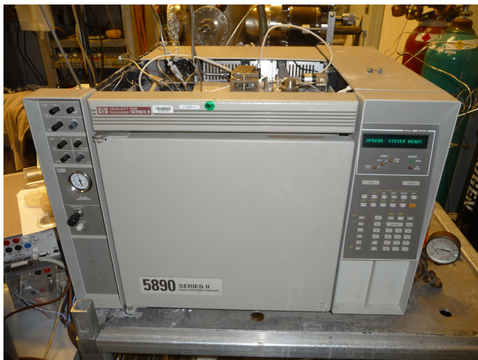
Figure 4.1 HP 5890 Series II Gas Chromatograph commonly used for kinetic measurements
