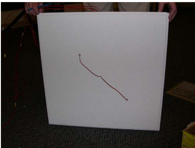
Figure 42: Ceiling panel surface sensors, room side
