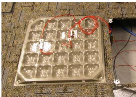
Figure 36: Temperature sensors in UF plenum
