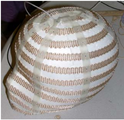
Figure 12: Manikin with heat tape on the head
