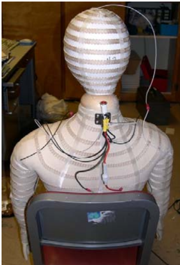
Figure 13: Assembled manikin sitting on chair from the back
