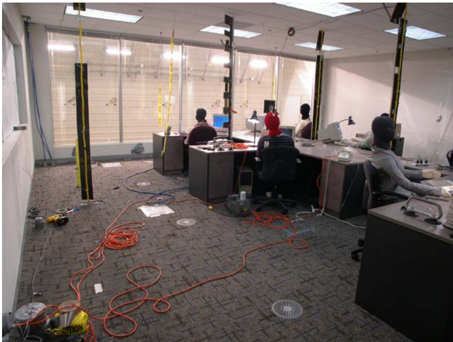
Figure 35: Test room view showing thermocouple trees with shielding
