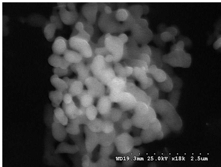
Figure 7.3: SEM image of LiFePO 4 powder made via the glycine nitrate combustion method. Secondary particles with a diameters in the range of 200-300 nm are comprised of ~30 nm primary particles.
