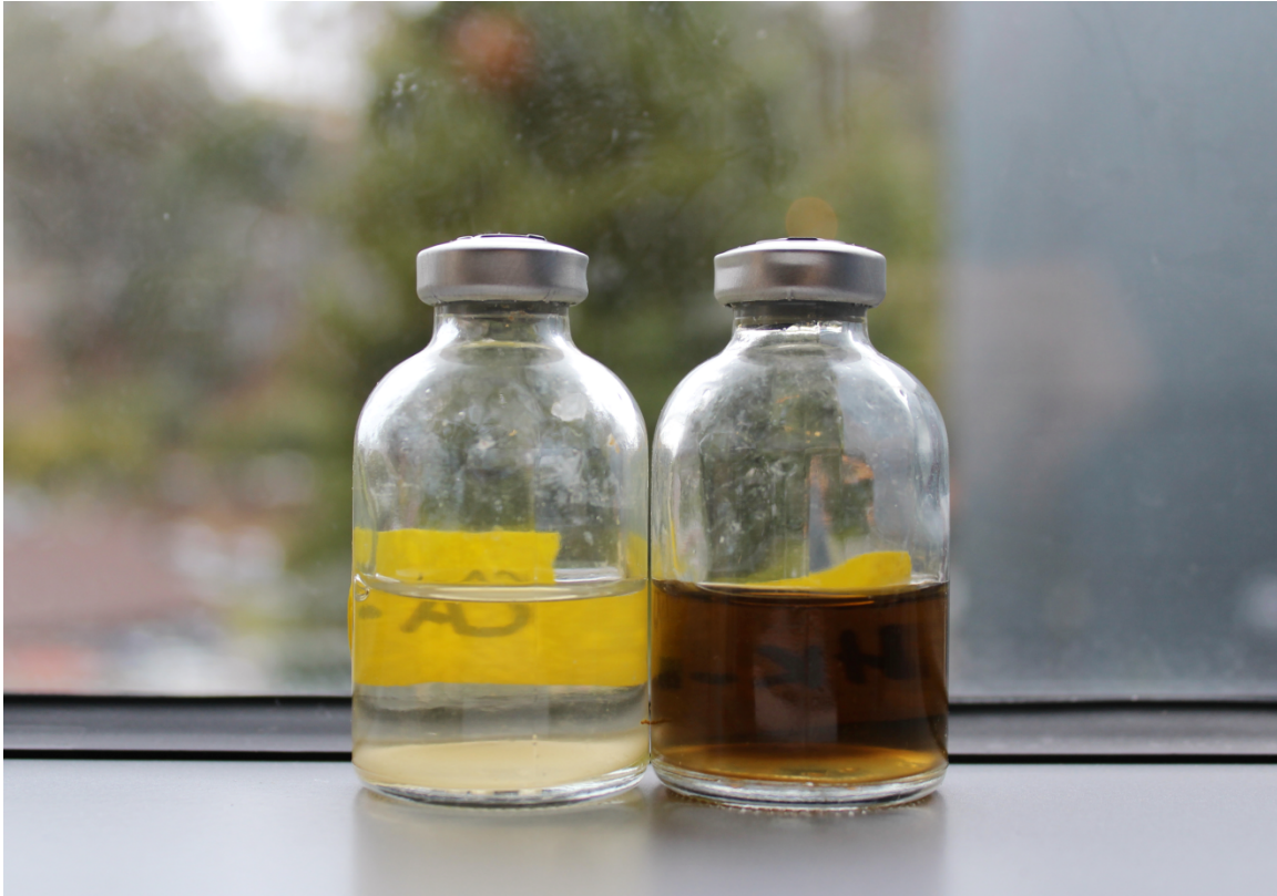
Figure 4-7. cymAmtrA was able to completely clear the Fe(III) citrate from the media. Clearing of Fe(III) citrate by the cymAmtrA culture (left) versus heat killed sample (right). None of the other strains described previously have ever shown complete clearing of Fe(III) citrate from the media.
