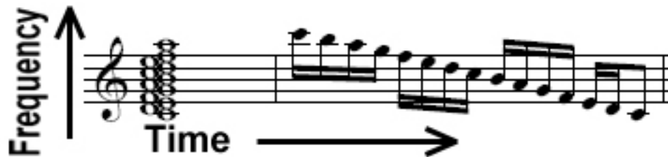
Figure 3.7: This is a music score that graphically represents a spectrograph function. The x-axis is time and the y-axis is frequency. The notes represent the intensity of the signals. There are two pulses shown in this spectrograph. The pulse on the left is a pulse with no chirp while the pulse on the right is negatively chirped .
