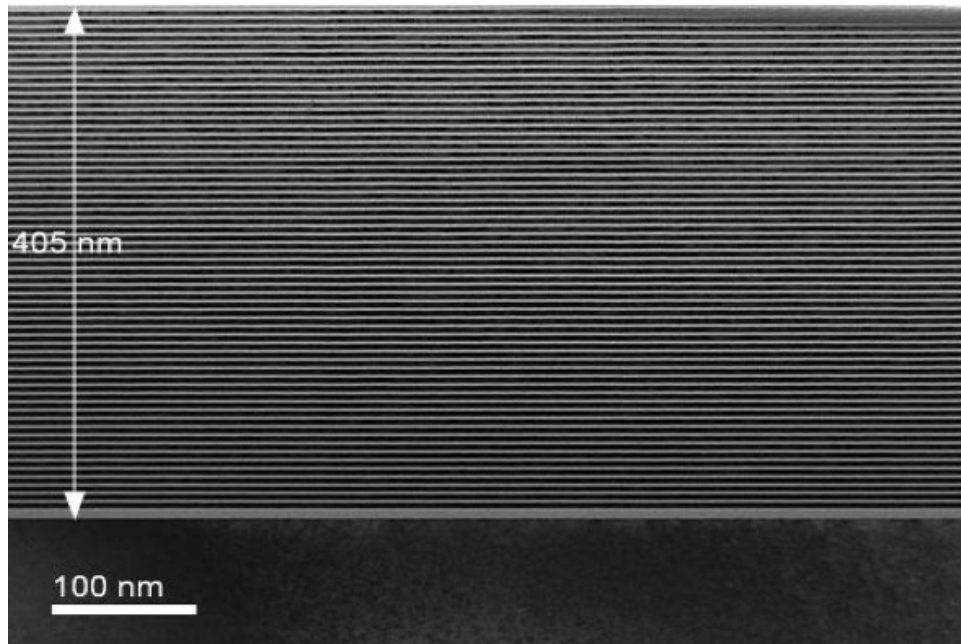
Figure 1.2: A cross-section TEM of a Molybdenum/Silicon (Mo/Si) multilayer. (Courtesy of E. Gullikson, Center of X-ray Optics)
