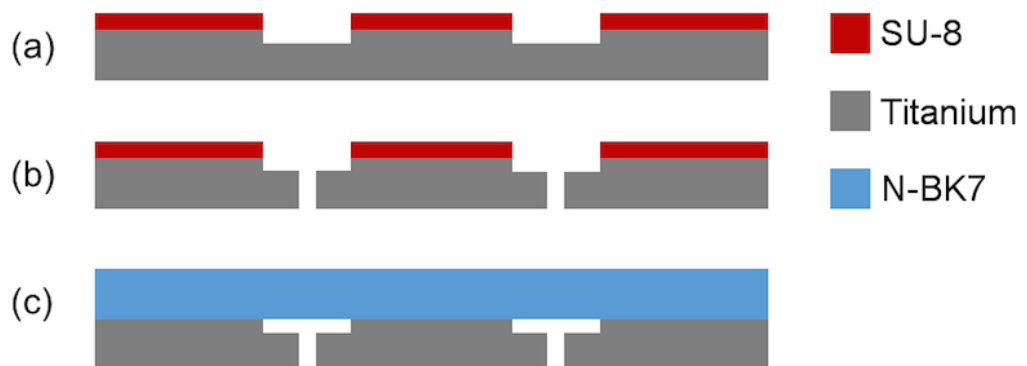
Figure 4-2. Fabrication process for burst pressure testing specimens: a) Lithographic patterning of Ti, followed by Ti DRIE to define micromachined fluidic reservoirs within the Ti substrate; b) Through-wafer via definition using manual milling to provide fluidic access to the reservoirs; c) Anodic bonding with N-BK7 substrate to seal the reservoirs.
