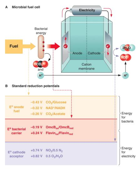
**Figure 2**. Bacteria use direct and mediated mechanisms to transfer electrons from the cell membrane to the anode surface. Electrons can be transferred from the cell or through a conductive biofilm using each method. References: Redox potential of *Shewanella* produced flavin (6) and a *Geobacter* (OmcB) outer membrane cytochrome (33).
