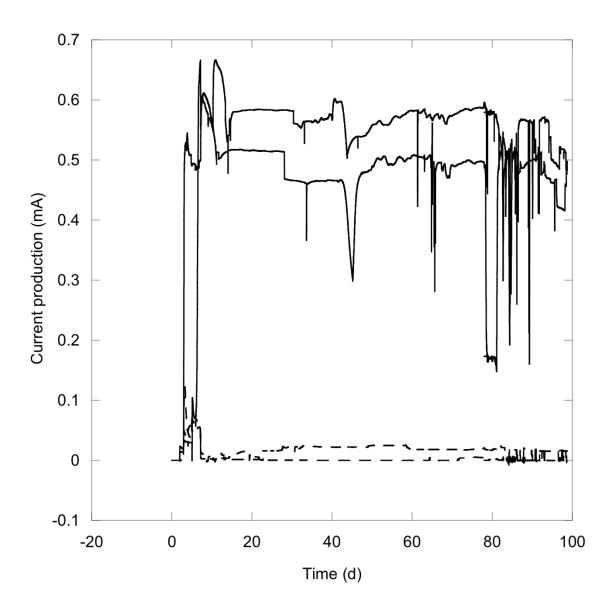
**Figure 4.** Current production by *Geobacter sulfurreducens* strain PCA in the H-type MFC used in this study. Cells were inoculated into anode containing growth medium (10mM acetate) and graphite block anode.
