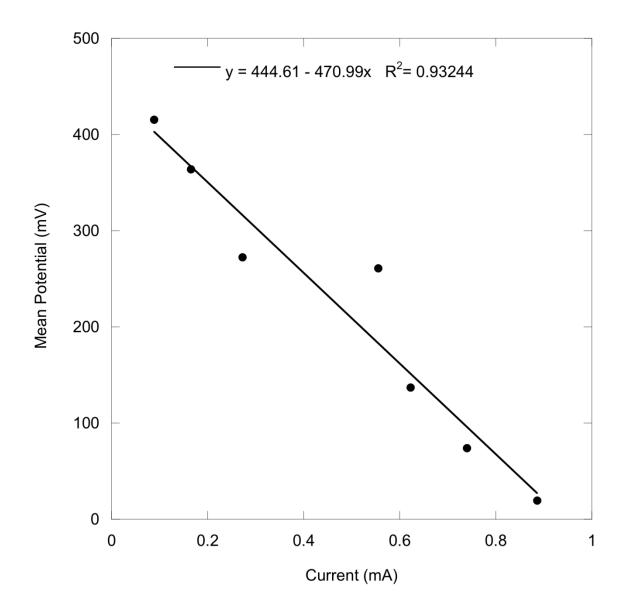
**Figure 8.** The current-power relationship is summarized in a power curve for thermophilic MFCs operated on acetate. The maximum short-term power (MPP) was approximately 0.15mW or 24 mW.m<sup>-2</sup>, while the maximum power for the experiment was 37 mW.m<sup>-2</sup>.
