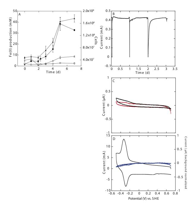
**Figure 4**. Fe(III)-oxide reduction by *Thermincola potens* strain JR incubated with 12 week old batch-operated MFC supernatants (80% v/v). Effects on the rate of iron reduction over time with the addition of 8mL of either supernatant (dashed line, o), fresh medium ( $\blacksquare$ ), 50  $\mu$ M AQDS and fresh medium (x), or fresh medium without acetate ( $\Box$ ) are shown.
