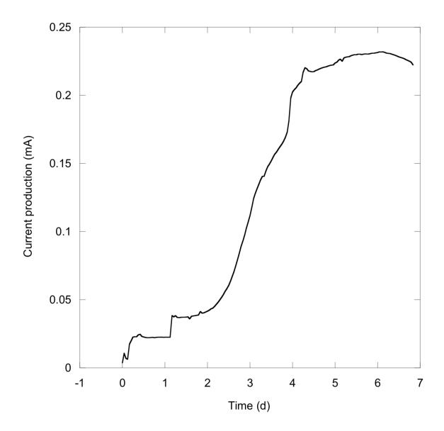
**Figure 5.** Coulombic efficiency is the ratio of total coulombs actually transferred to the anode from acetate to the maximum possible coulombs if all acetate removal produced current. The total coulombic yield from acetate oxidation is determined by integrating the current over time. Of the 82.3 C added as acetate, a mean of 73.1 C could be recovered as current, indicating a recovery of 89%.
