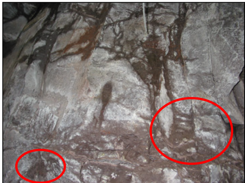
Figure 8. Development of lateral flow along the back wall of Niche 3 over a period of 24 hours. This wetting likely occurred as water was diverted from the ceiling migrated through the formation close to the walls. Circles indicate the location of changes.
