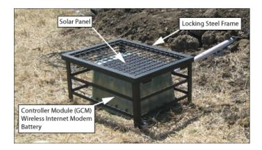
Fig. 4. Remote monitoring station.
