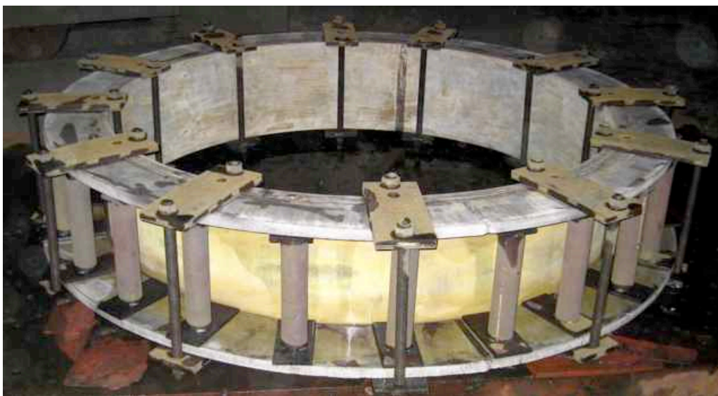
Figure 16. The rough coupling coil mandrel as prepared for heat treatment before machining.
