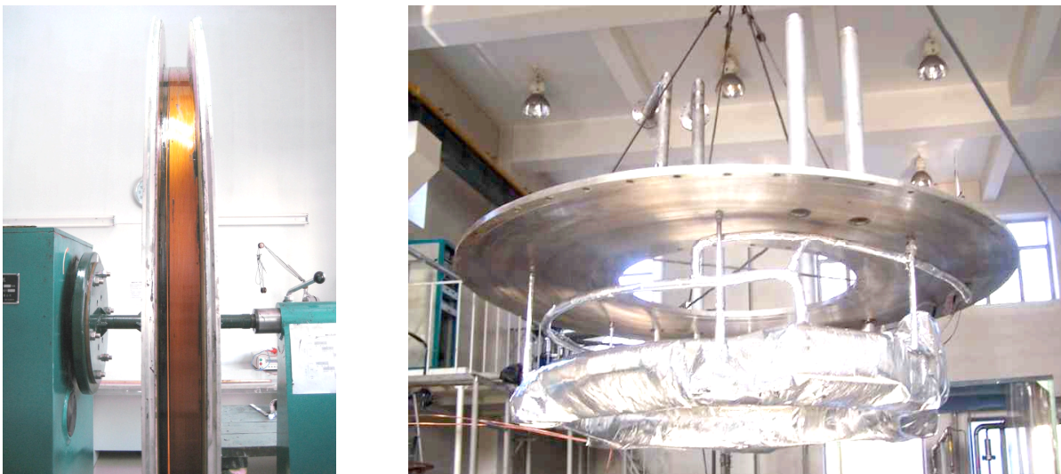
Figure 15. The large ICST test coil. (Left, the large test coil is being wound on the ICST winding machine. Right, the insulated large test coil is being lowered into the large ICST vacuum chamber.)
