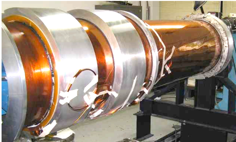
Figure 8. The winding of spectrometer magnet one (summer 2007).
