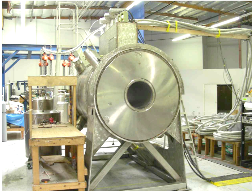
Figure 10. The finished first spectrometer solenoid during the magnet test (July 2008).
