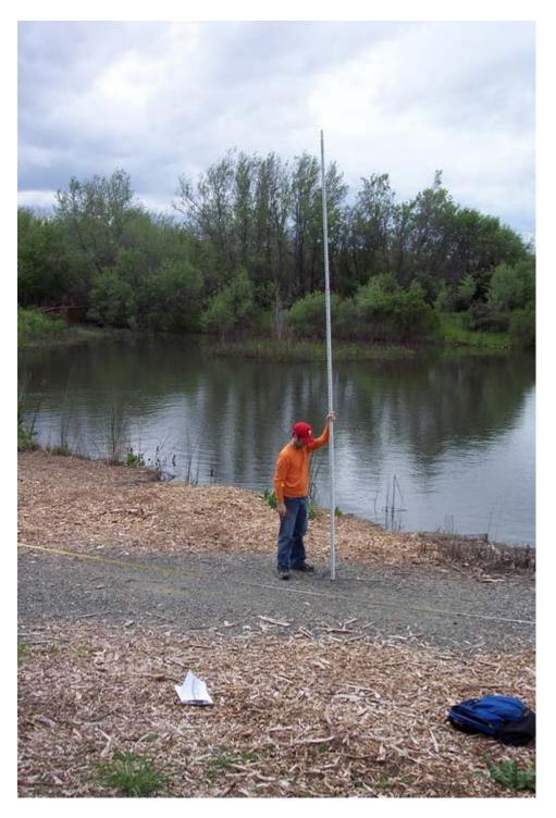
Photo 3. Typical land survey procedure measuring elevation of features such as the road. Pond C Island 2 in the background which is just below water level at the time of sampling.
