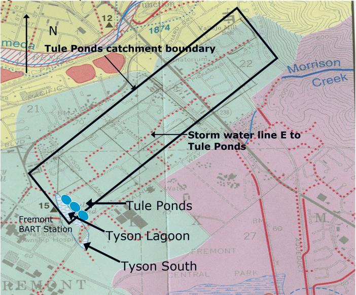
Figure 3. Detailed engineering plans with location of cross sections, water samples, and indented flow. Outflow leads to Tyson Lagoon, which is due west of the Tule Ponds.
