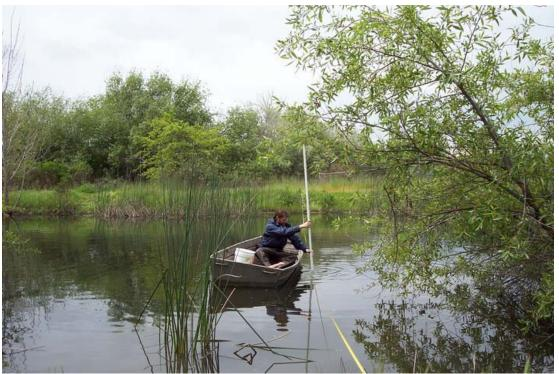
Photo 2. We conducted cross section measurements along a fixed transect line using a row boat. This proved to be challenging, especially when winds were high.
