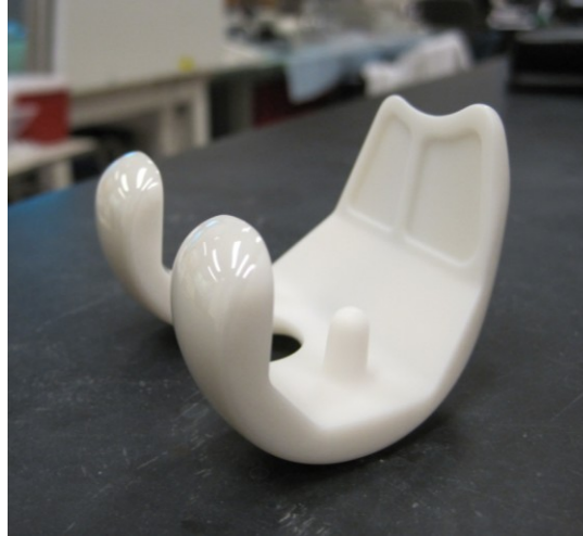
Figure 5.1-1. Photograph of the as-received commercial zirconia femoral knee implant.
