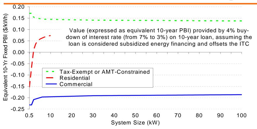
PBIs for 7% and 3% loan cases calculated to be equivalent, on a customer-NPV basis, to a \$2.8/W CBI. Graph shows difference between PBI in the 3% loan case to the PBI in the 7% loan case. Both cases assume – aggressively – that the entire capital cost of the project is financed with the loan in question.
