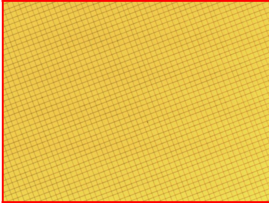
Figure 4.8. Optical image of a grid pattern with controlled 50- \mu\text{m} spacing from an area highlighted by the red box in Figure 4.7.
