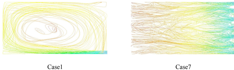
Figure 6.11: The flow patterns for Case 1 and 7 ( Q=0.02\text{m}^3/\text{s} , buoyancy included)
