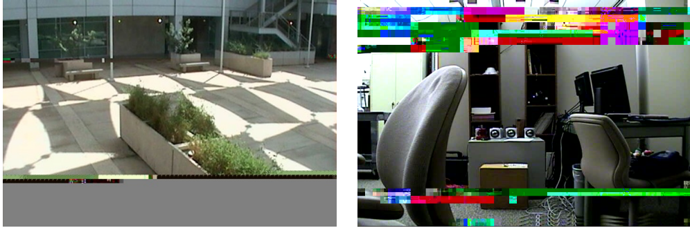
Figure 2.2: Stream corruption caused by network congestion may manifest in different ways depending on the video format. Left: corrupted Motion JPEG stream due to partial data, right: corrupted MPEG-4 stream due to partial data.
