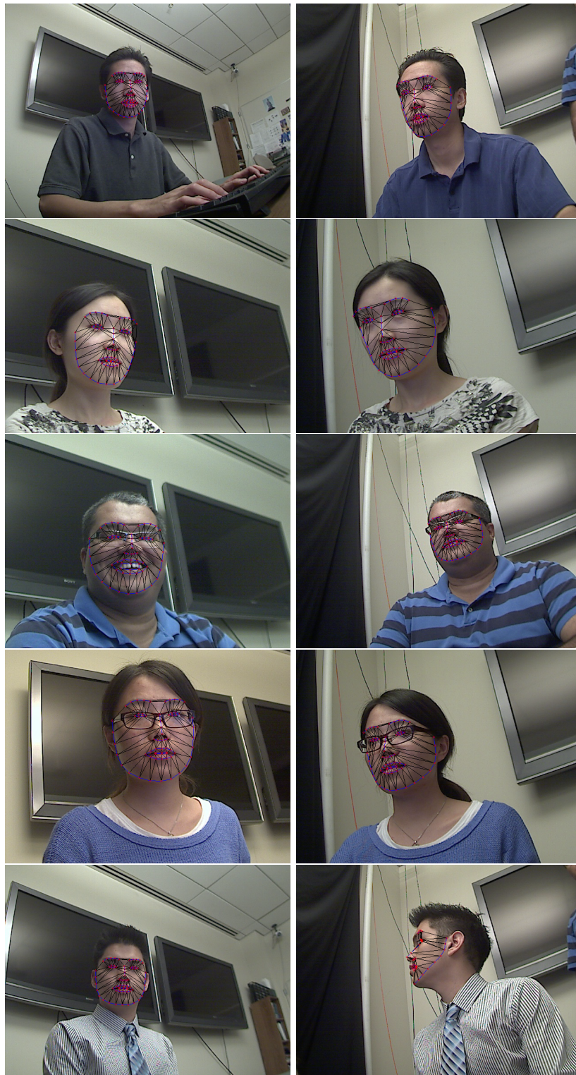
Figure 6.2: Automatic landmark detection done in real-time using Constrained Local Models (CLMs).
