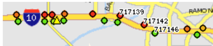
Figure 33: From the PeMS website, an image demonstrating the irregular placement of ILD on the Los Angeles freeways. ILD are not equally separated along the highways, which is not a bad thing. The density of ILD is higher along busier sections of the f
