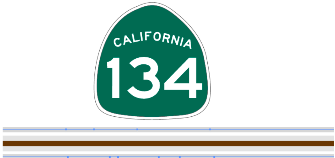
Figure 33: From the PeMS website, an image demonstrating the irregular placement of ILD on the Los Angeles freeways. ILD are not equally separated along the highways, which is not a bad thing. The density of ILD is higher along busier sections of the f
