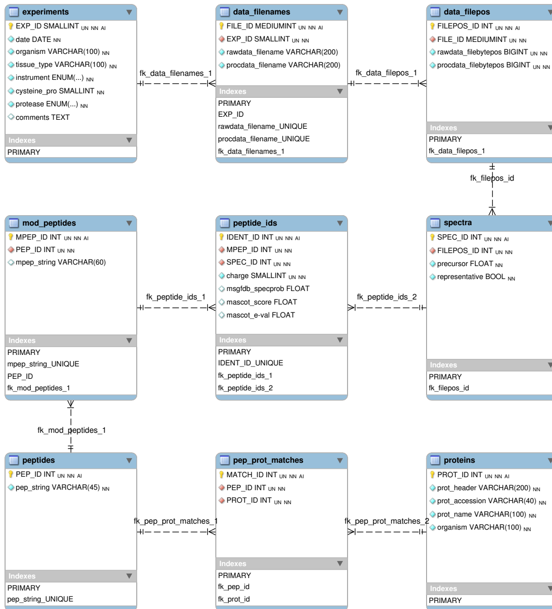
Figure 5.1: Database model for spectral library. All spectra were inserted in the database, allowing user to search against both identified and unidentified spectra.
