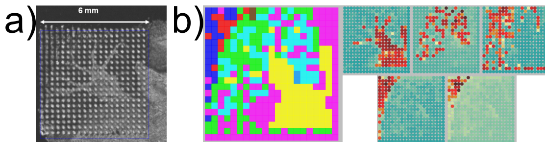
Figure 5.2: AMASS results for MSI data. a) optical image with MALDI spots. b) (left) segments resulting from an AMASS run with random seeds after 3 iterations. (right) log-odds images for the AMASS segments. We can see the different regions of the cerebellum.
