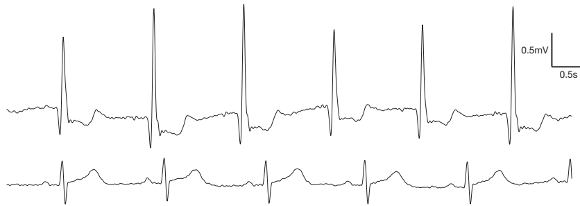
Figure 6.8: Artificial (top) and live ECG (bottom) signals acquired by the BioADC. Passive AgCl clinical adhesive electrodes on the subject’s were connected directly to the BioADC’s inputs. The subject was also passively connected to circuit ground through a third AgCl electrode.
