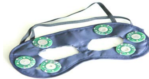
Figure 7.3: Bio-cursor head-mask with six EOG electrodes.
