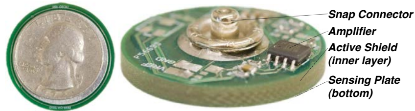
Figure 4.2: Picture of the non-contact, non-contact electrode. The sensor is manufactured on a standard PCB, which contains the amplifier circuits on the top and the sensing plate on the bottom.
