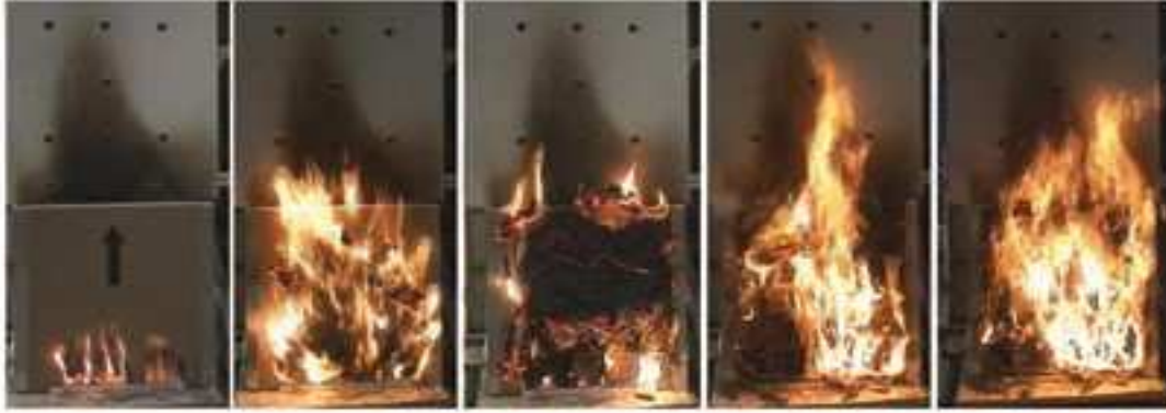
Figure 5.2: Test 2 Timeline: (a) 21 seconds, laminar burning on front face, (b) 50 seconds, front layer of cardboard burned off; cardboard in bottom two rows of cells ignited, (c) 70 seconds, PS cups melted earlier than other tests, melted to front face and created shield stalling burning rate, (d) 122 seconds, bottom row of cups ignited, forcing top layer of cardboard/melted PS off, (e) 172 seconds, entire front layer of PS cups and cardboard burning in wall. Second layer of cells beginning to ignite.
