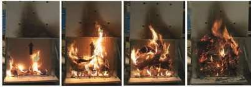
Figure 5.1: Test 1 Timeline: (a) 53 seconds, peeling front face of cardboard, (b) 75 seconds, 1st layer cells cardboard ignite, (c) 89 seconds, PS cups in bottom row of first layer begin to deform, (d) 113 seconds, all PS cups and cardboard in 1st layer engulfed in flame.
