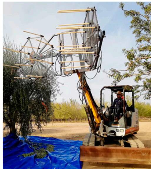
Figure 4. The shaker header is attached to the retractable boom of a Bobcat 337.
