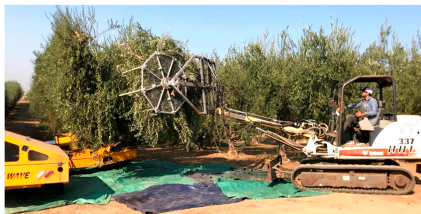
Figure 6. Trunk shaker and canopy shaker, shaking an olive tree simultaneously.
