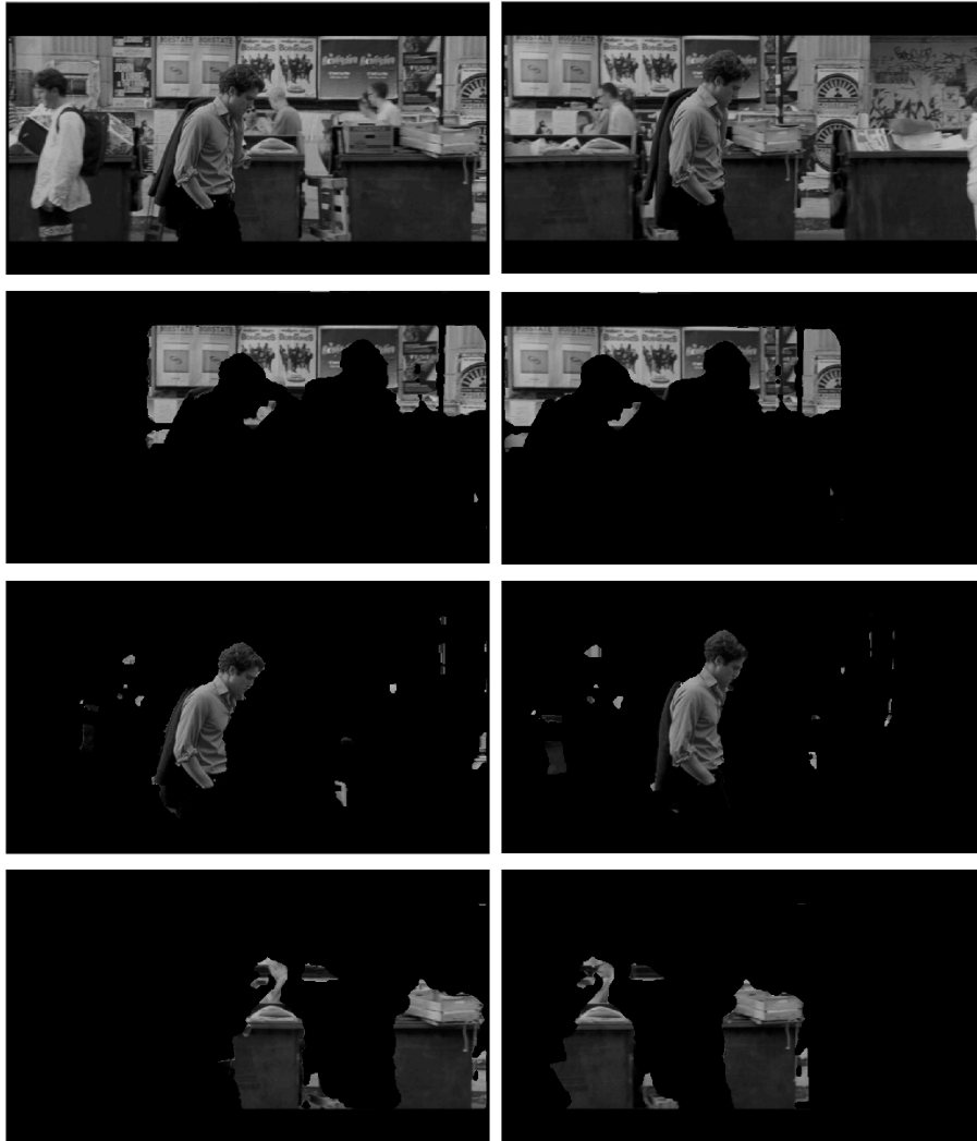
Figure 2.6 Notting Hill sequence. (Row 1) Original image pair of size 311 \times 552 , (Rows 2-4) Pixels assigned to warp layers 1-3 in I and I' .
