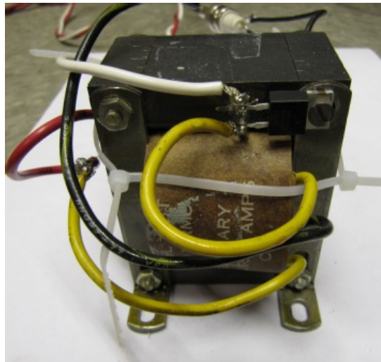
Figure 5.9. The transformer used for solving the issue of current transients in the earth field cancellation coil due to polarizing pulses.
