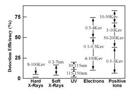
**Figure 2-5.** Detection Efficiency of Charged Particles and Electromagnetic radiation in MCP detectors. (Netolicky 2009)
