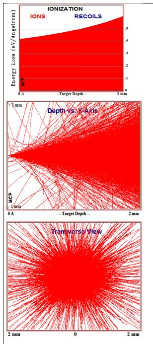
**Figure 2-15.** 25 MeV Proton Interaction with MCP. (Top Panel) Energy Loss vs. Depth. (Middle Panel) Ion Tracks vs. Depth – Cross Section. (Bottom Panel) Transverse – "Anode View" – of Ionization Tracks in MCP.
