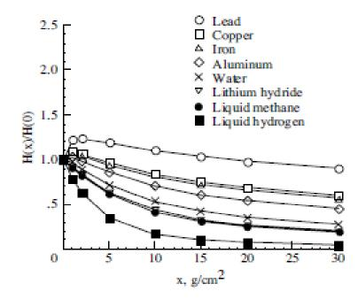
**Figure 5-10.** Attenuation of dose equivalent for a one-year GCR exposure at solar minimum behind various shielding materials. Material Densities (g/cm<sup>3</sup>): Lead = 11.35, Copper = 8.96, Iron = 7.87, Aluminum = 2.70, Water = 1.0, Lithium Hydride = 0.82, Liquid Methane = 0.42, Liquid Hydrogen = 0.07. (Wilson et al. 1999)
