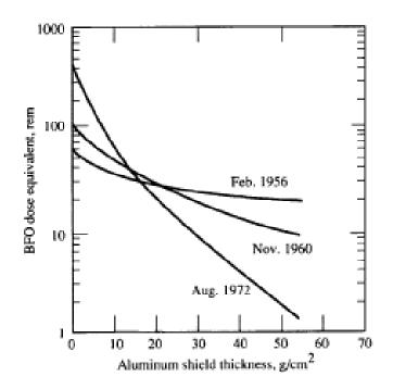
**Figure 5-9.** Blood forming organ (BFO) dose equivalent as a function of aluminum shield thickness for three large SPE's.  $1 \text{ g/cm}^2$  of aluminum is equivalent to 0.37 cm thickness. 1 rem = 10 mSv. (Simonsen and Nealy 1991)
