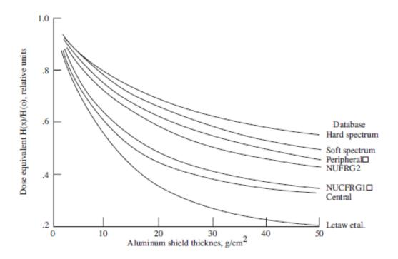
**Figure 5-8.** Shield attenuation for solar minimum galactic cosmic ray dose equivalent resulting from nuclear fragmentation models. 1 g/cm<sup>2</sup> of aluminum is equivalent to 0.37 cm thickness. (Wilson et al. 1999)
