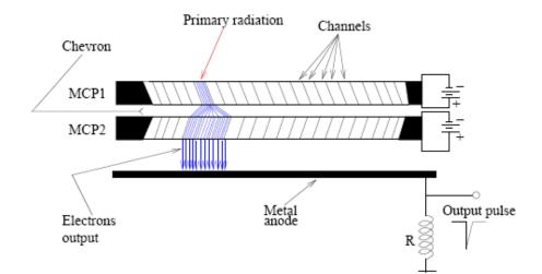
Figure 2-4. Chevron Configuration for MCP Detectors. (Kosev 2007)
