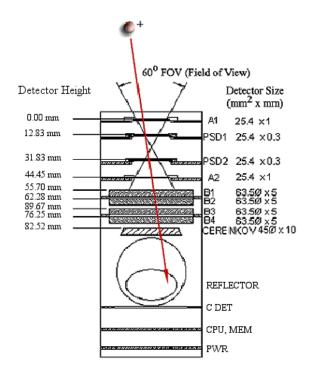
Figure 2-17. Schematic of MARIE detector stack. (Pinsky and Wilson 2002)
