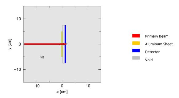
**Figure 2-9.** Geometric model used in PHITS to determine the flux of secondary particles from SEP's traversing 3mm of aluminum. (Image generated by PHITS)
