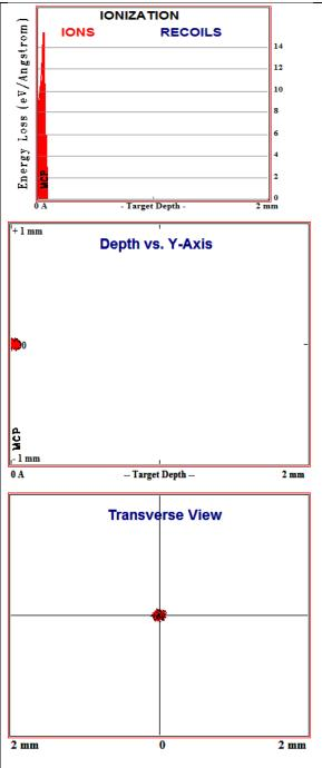
**Figure 2-14.** 8.25 MeV Helium Interaction with MCP.(Top Panel) Energy Loss vs. Depth. (Middle Panel) Ion Tracks vs. Depth – Cross Section. (Bottom Panel) Transverse – "Anode View" – of Ionization Tracks in MCP.
