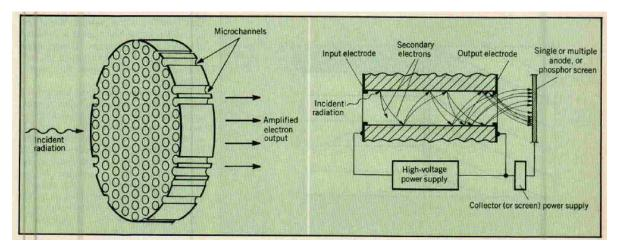
Figure 2-3. Operation of a typical MCP detector. (Leskovar 1977)
