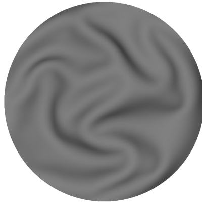
Figure 5.3: Top view of the membrane deformed configuration at t = 0.15 s. Despite the complex deformation pattern, the wrinkles on the membrane surface are smooth.
