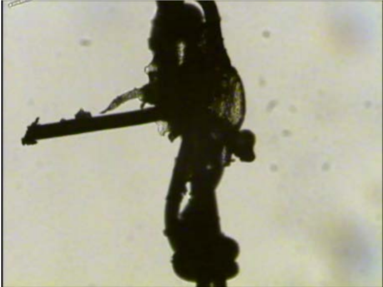
Figure 9.4. A magnified view of a modified Albright knot splicing two platinum wires together. The magnification is 100x.
