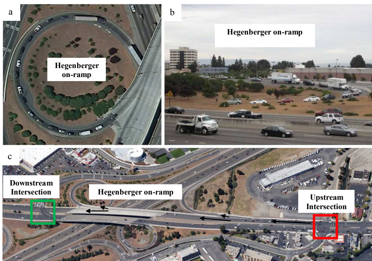
Figure 3.1: Photos showing (a) aerial view of Hegenberger on-ramp with saturated queue, (b) side view of Hegenberger on-ramp with saturated queue, and (c) arterial streets and intersections around Hegenberger on-ramp
