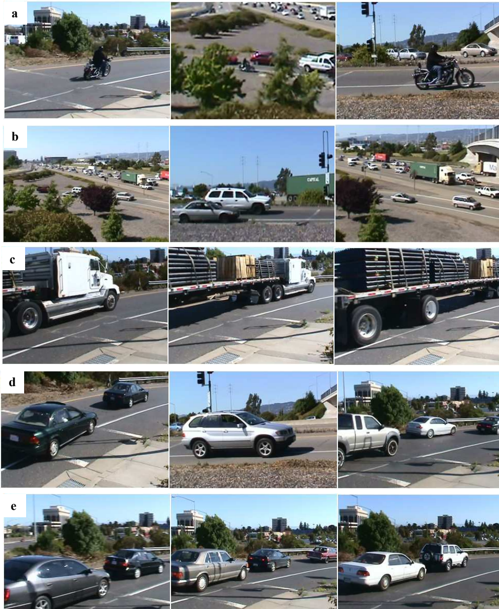
Figure 3.13: (a) Motorcycle bypassing queue, (b) vehicle bypassing queue, (c) large truck entering on-ramp, (d) off-centered vehicles with respect to lane, and (e) adjacent vehicles simultaneously stopped on top of leading and trailing speed-trap sensors
