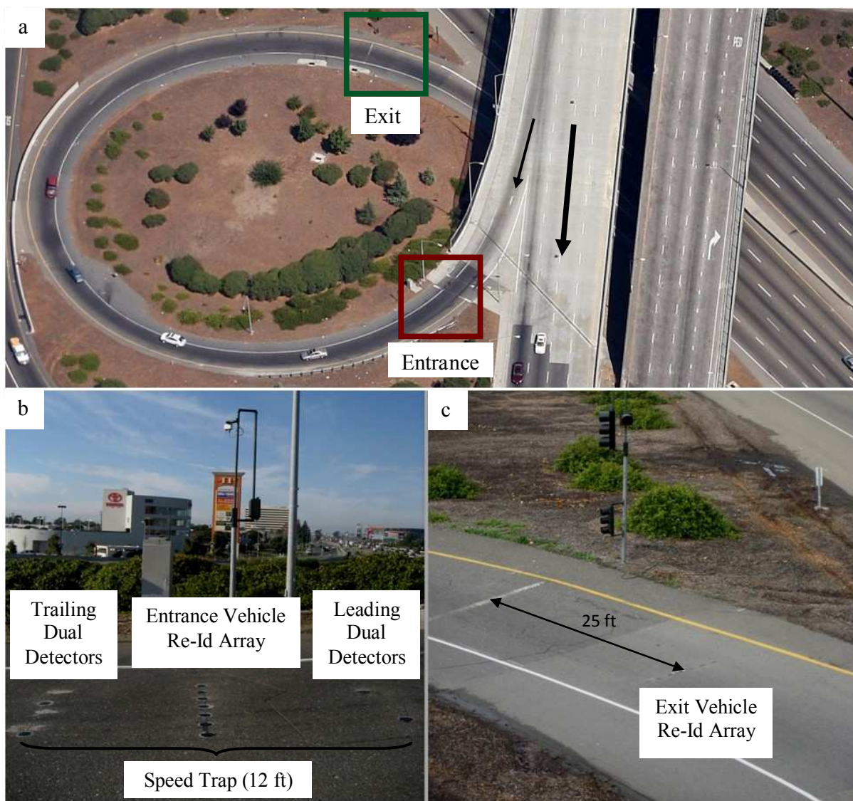
Figure 3.3: Photos showing (a) Hegenberger on-ramp entrance (bottom square) and exit (top square), (b) vehicle detection system installation at ramp entrance, and (c) sensor array installation at ramp exit (Re-Id = re-identification)
