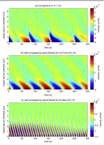
**Figure 6.** Space–time diagrams showing the time evolution along the vertical line at x = 11.7 cm of the horizontal velocity field measured by PIV in the stratified zone (see the corresponding movie 'InternalWaves.avi' in the supplementary material). As in figure 5, (a) shows the full signal, while (b) and (c) show the corresponding signals including right-propagating waves only, filtered around the frequency f = 0.013 Hz and f = 0.06 Hz, respectively.
