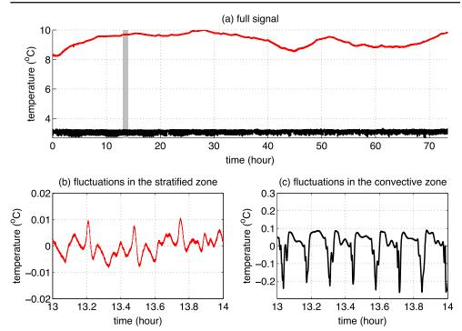
**Figure 2.** (a) Temperature measurements during 3 days at fixed locations in the convective zone (lower black signal) and in the stratified zone (upper red signal) as a function of time in hours. (b) and (c) show a zoom of the corresponding fluctuations between 13 and 14 h—shown by the gray rectangle in (a)—once secular trends have been removed by a polynomial fit.
