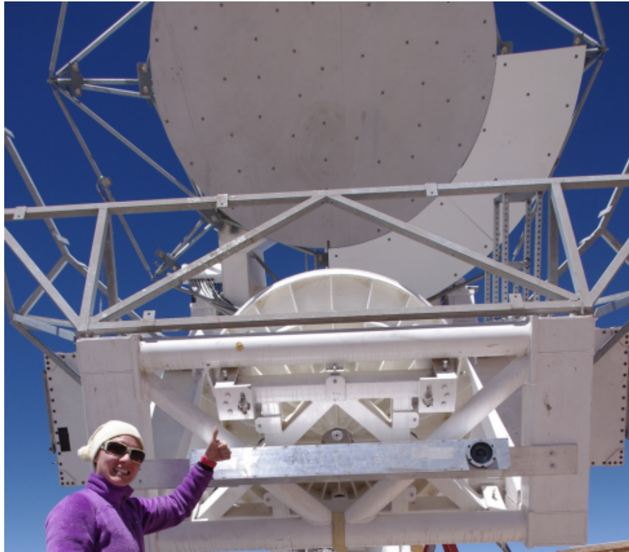
Figure 3.12: The star camera mounted to the telescope during assembly in Chile, with me in the foreground. The star camera is attached to the forward most component of the telescope boom through two extension pieces of aluminum. The primary and secondary mirrors can be seen in the background.
