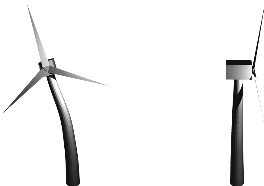
Figure 2.17: Frontal and side views of the 1 st side-to-side bending mode at the peak of acceleration response. (forced-harmonic result)
