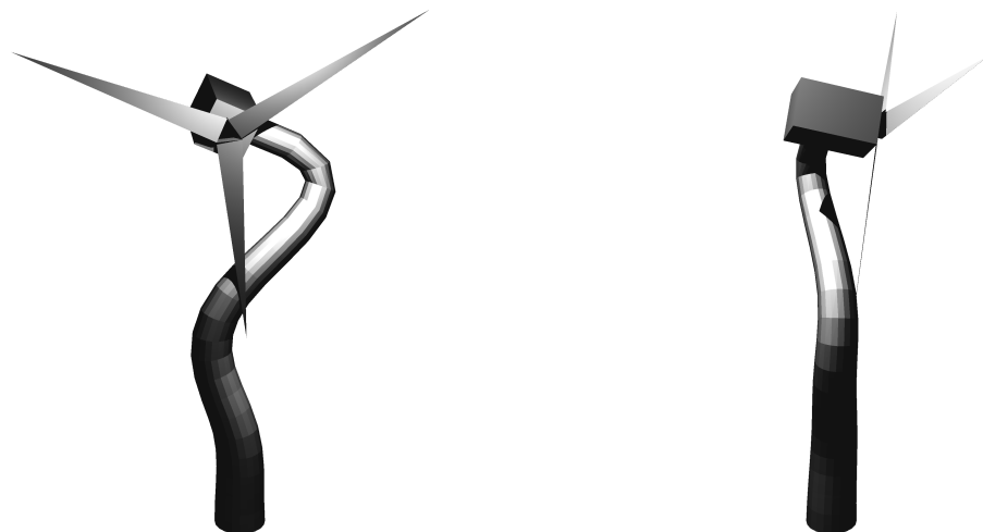
Figure 2.21: Frontal and side views of the 3 rd side-to-side bending mode at the peak of acceleration response. (forced-harmonic result)
