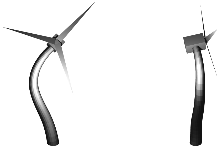
Figure 2.19: Frontal and side views of the 2 nd side-to-side bending mode at the peak of acceleration response. (forced-harmonic result)
