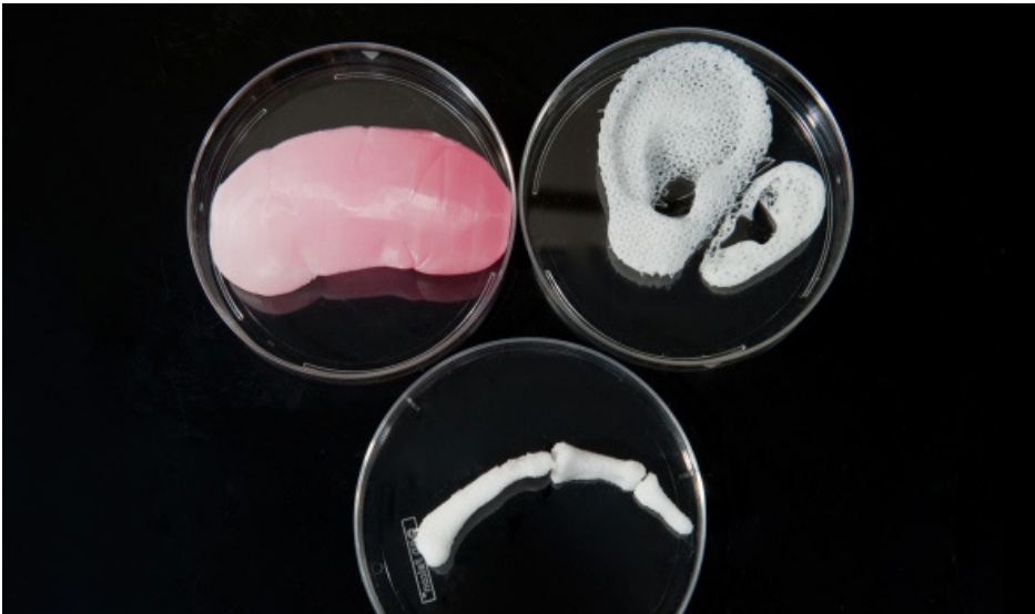
Successfully 3D printed bone, ear, and kidney prototype, from Wake Forest Institute of Regenerative Medicine
